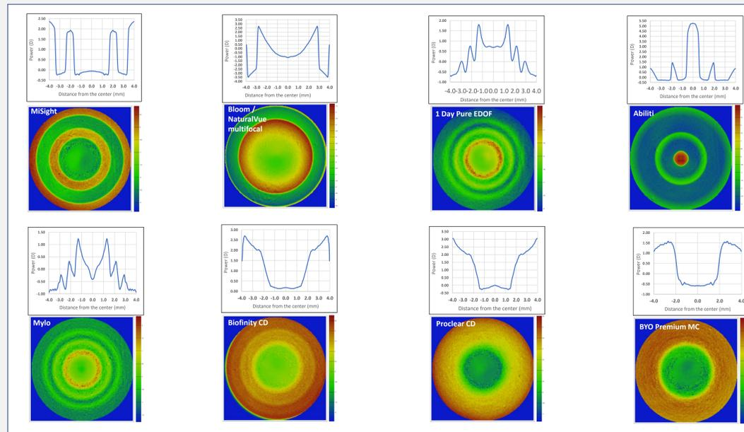
Figure 1. Radial power profile and color power map of lenses analyzed; for a better comparison between different designs the radial power profiles were plotted removing the labelled lens power from the raw data.
